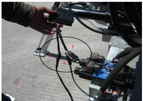
12. Tighten four pcs of oil pipes. Pipe a and c shall be the upper. 13. Tighten inlet and outlet oil pipes. Connect power.12.13.14.
