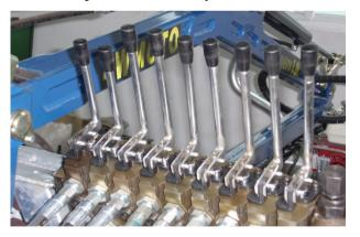
Pressure of relief valve is 10Mpar~12Mpar. Please adjust relief valve or increase engine speed for compression to lift heavier weights. Relief valve is in right sight of multi-control valve. Take away the cap, there is A-folt bolt. Clockwise is adding to pressure, Anticlockwise is reducing pressure.
